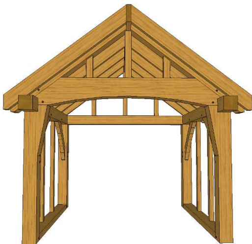
ref 2537 (finishing required on-site) 2.25 (w) x 2.00 (d) x 2.52 (h) - posts 145x145mm
